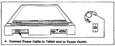
5. Turn the 2500 tablet ON. The power switch is next to the power cord at the rear of the tablet. 0 is off, and 1 is on. The tablet will run a series of self-tests and then beep to indicate it is ready. If the TEST light is flashing after power up, see page 42.
